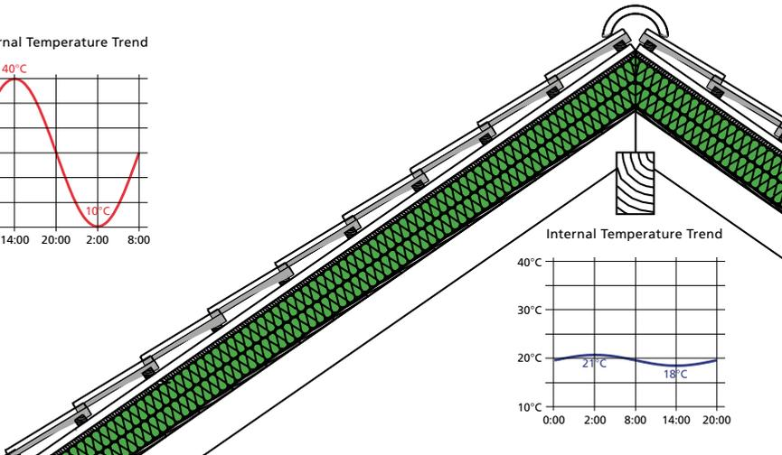
Amplitude Dampening and Phase shifting are as vital for summer heat protection as the U value is for Thermal insulation in winter. Amplitude Dampening shows the strength with which the temperature penetration is reduced. The Phase Shift shows, by how many hours, the penetration of the maximum temperature is delayed.
