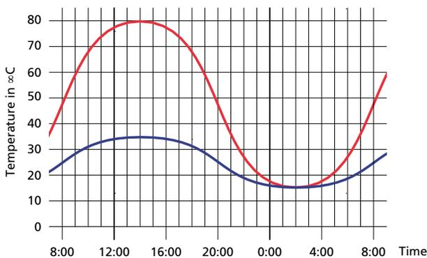
Temperature under the roof covering
