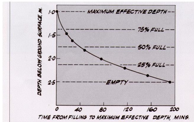
Figure 2 Field observations from a soakage trial pit
