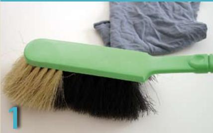
All surfaces must be stable, dry, smooth and free of dust, silicone and grease. Sweep or vacuum clean and wipe all surfaces.
