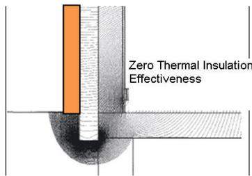
In the second drawing, the insulation has been lowered by 40cm. This simply makes the passage of heat more difficult.
